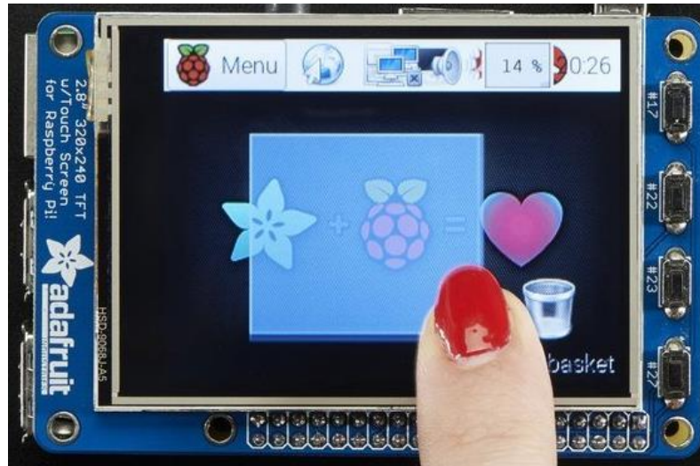
Figure 22: Adafruit PiTFT 2.8" Touchscreen
