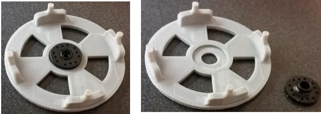
Figure 41: Left: Driver ring with servo horn, Right: Driver ring without servo horn
