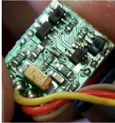
Figure 22: Burnt transistors on the internal servo driver board
