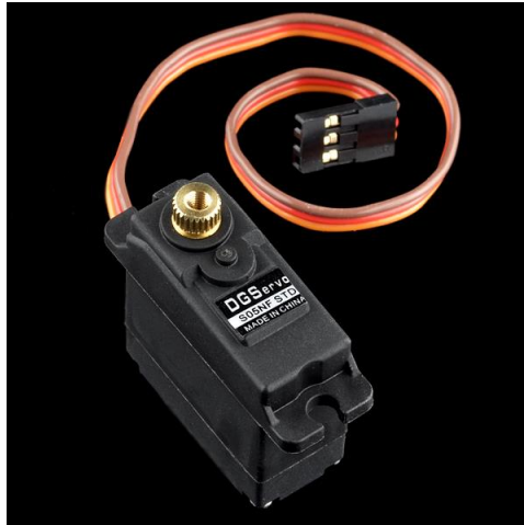
Figure 39: Servo used in the drone coupler system
