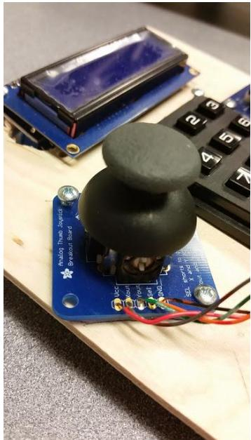
On the controller side again, the LCD screen was set up in a way to allow the user to see important information about which mode they were currently in or values that were of interest to them. This was done using an updated version of the LiquidCrystal Library that allowed communication over I2C. A good reason to make this over I2C is to allow more pin availability for things like the keypad and other devices, otherwise 7 or more pins will be taken for the screen alone.
