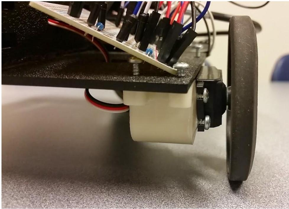
For the continuous servo finding the center position, where the wheels no longer move is preferred first. Finding the approximate top speed in both directions if found using the same process as before, but this time watch until the servo appears at top speed or starts making strange noises and scale back the values. Place the new servomax and servomin values into the
