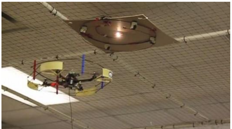
Fig. 4. Demonstration of bottom up wireless power transfer.
