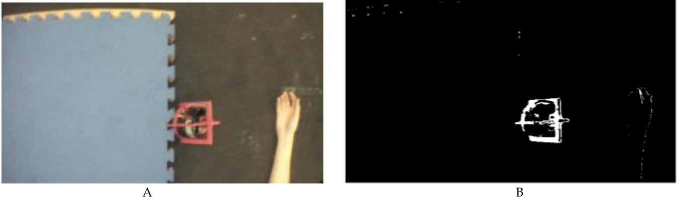
Fig. 16. A sensor node passed through the color filter, A is the original image, B is the output of the color filter.
